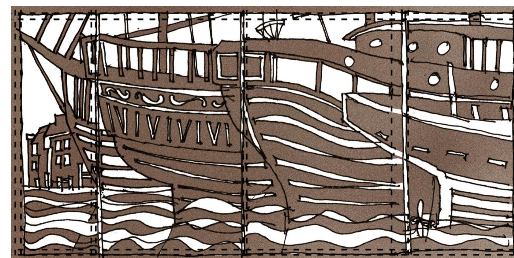
Gate artwork laser cut in 6mm thick steel sheet and welded on existing gate
